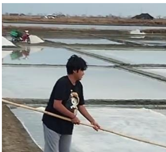
Figure 2. Documentation of the salt “raking” process in the ponds of Asempapan Village
